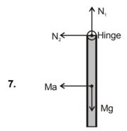
Initially rod is at rest So,  $N_1 = Mg$ ,  $N_1 = Mg$ Torque = I $\alpha$
